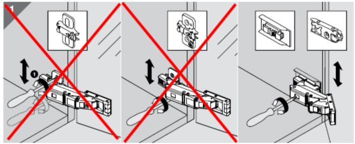
Use the center screw to adjust the vertical alignment of the door. To gain access, open the door to approximately a 45° angle or until you can see the center screw through the square opening in the hinge as shown above.
