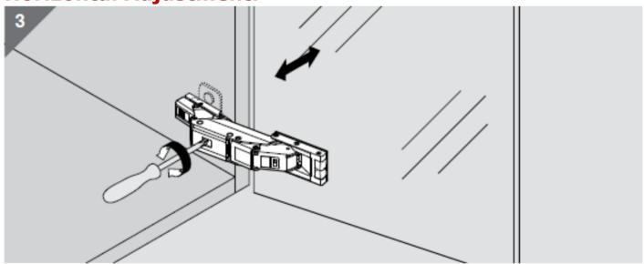
Use the screw at the front of the hinge (closest to the mirror door) to adjust the horizontal alignment of the door. You can access it by having the door open at a 90° angle and placing the driver through the square hole in the hinge as pictured above.
