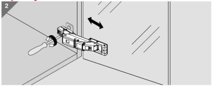
Use the screw at the back of the hinge (closest to the back of the cabinet) to adjust the depth alignment of the door. You can access it by having the door open at 90° angle as pictured above.
