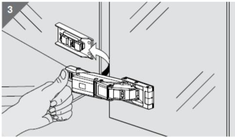
With the hinges all in their open position, pick up the door and attach all hinges to the base plate in the cabinet frame as shown above in the picture above. If done properly, you will hear a "click" sound. Ensure this is done for all hinges in the cabinet.
