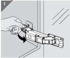
Place your hand at the back of the narrow part of the hinge. Here you will find a small tab in which you will pull inward (towards the inside of the cabinet). This will release the hinge from the cabinet (hinge plate). Do this step for all hinges before proceeding.
