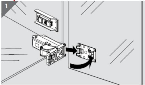
Ensure all hinges are in the closed position creating an "L" shape. Then attach the hinge to the door as shown above.
