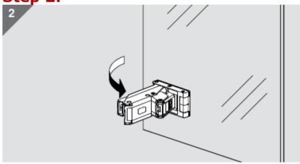
Once all hinges are released, they will remain attached to the mirror door. Carefully place the mirror door on a clean, flat surface. Then "close" the hinges as shown above and proceed to step 3. Page 5
