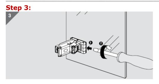
Using a flat head screw driver in one hand and holding the hinge with your other, carefully insert the flat head between the hinge and the plate attached to the mirror door. Then turn your driver to lift the clip that attaches the hinge to the hinge plate on the mirror door until it releases. Please be sure you're holding the hinge so it does not fall onto the door and cause damage.
